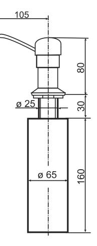
mm, maximum installation depth 30 mm, capacity 0.45 l, packed in a box
