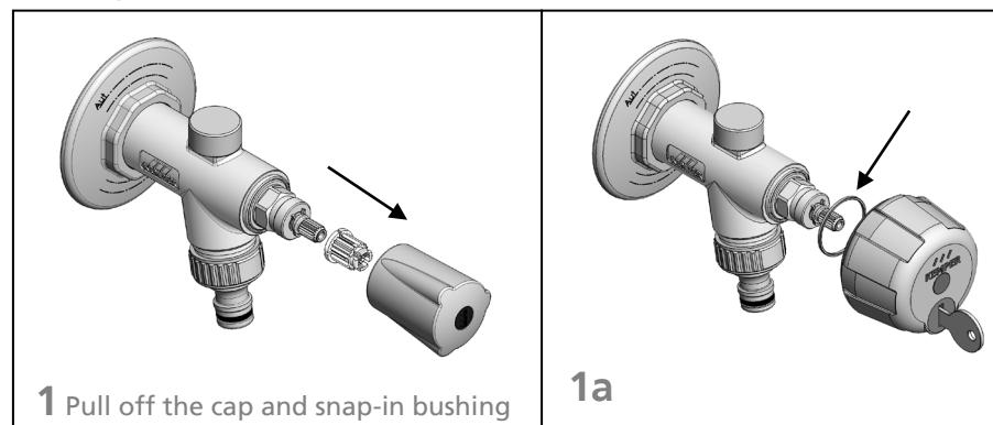
1 Pull off the cap and snap-in bushing
