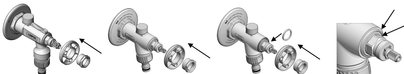
Attach the rear part of the handle A assembly and screw the threaded bush B onto the valve cartridge (torque 10 – 15 Nm). The rear part of the handle A should be easy to turn, without too much axial clearance (max. 0.3mm)
