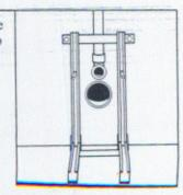
The inlet sleeve must protrude from the wall by 70 mm and the screws by 65 mm. The outlet should be fitted flush with the raw wall, at most with the finished tiled wall. The WC connecting sleeve must be fitted individually.
