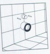
We recommend applying white cement to the rear of the WC to compensate for any unevenness. Grease may be applied to the wall surface to facilitate subsequent dismantling. Mount the WC and WC-seat and cover. Check the WC for water tightness.
