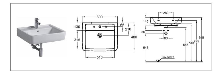
Rectangular wash basin, EN 14688 CL 25, made of sanitary ware porcelain With tap hole middle open, can be drift-punched at right and left with cleaning-optimised, inward-tilting bowl design
