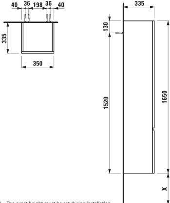
X = The exact height must be set during installation.
