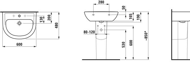
\* = Effective height must be fixed according to the height of the pedestal.
