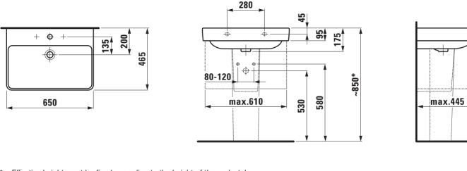
\* = Effective height must be fixed according to the height of the pedestal.
